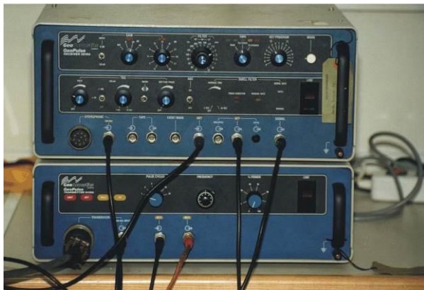
Figure 17: Receiver and transmitter (GeoAcoustics Ltd. GB) devices used as deck units for controlling the 3.5kHz acoustic signal.
