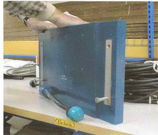
Figure 10: Hydrophone of the SeaBeam 2120 multi-beam system.
