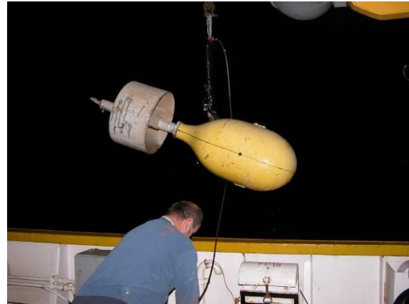
Figure 16: Deployment of the 3.5kHz sub-bottom profiler tow fish over the left side of R/V AEGAEO during the Farasan cruise.
