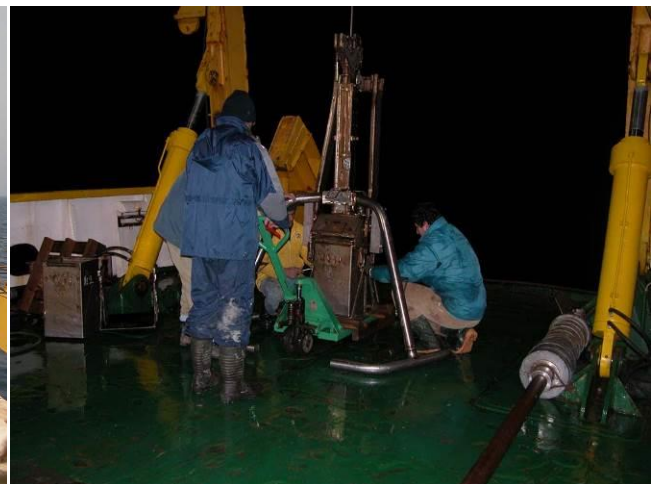
Figure 23: Box corer deployed through the A-frame at the stern of R/V AEGAEO in the Farasan area.
