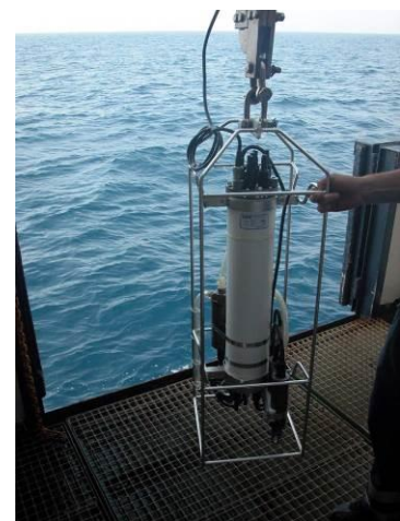
Figure 14: Sea Bird E-9 CTD system used during the Farasan cruise for measuring the sound-velocity profile of the water-column.
