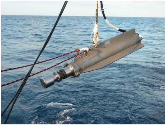
Figure 20: Deployment of Air Gun tow fish from the stern of R/V AEGAEO
