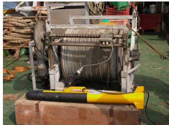
Figure 18: Side scan sonar tow-fish and tow-cable winch on the working deck of R/V AEGAEO during the Farasan cruise.
