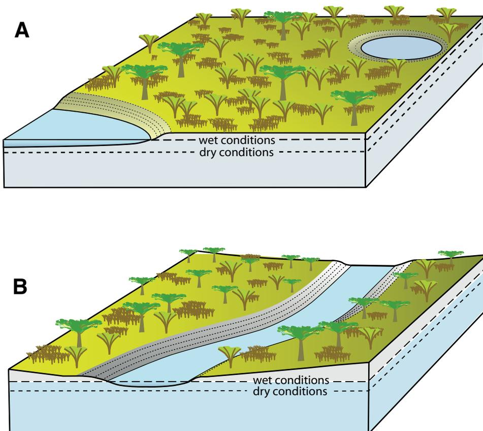
Figure 6. Schematic illustration of effects of changing water table in flat landscapes. (A) In regions of low relief, pans, water holes, and lakes are sensitive to changes of climate and can become dry if the water table drops. (B) Rivers in regions of low relief are also sensitive to changes of water table resulting from climate change and can be perennial or completely dry. If there is a reliable source of water from a high rainfall headwater region, such rivers can be more reliable.
