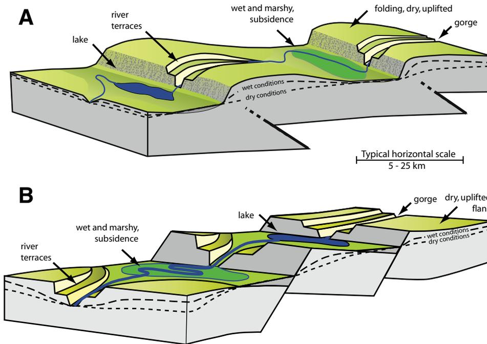
Figure 5. Schematic illustration of the effects of tectonic activity creating landscape features illustrated by examples in this paper. (A) Features typical of contractional (reverse-faulting) environments, where the surface expression of faulting appears in the form of folds as well as faults that cut the surface. (B) Features typical of extensional (normal-faulting) environments. These produce similar features as in A, but the faults usually fully cut the surface.
