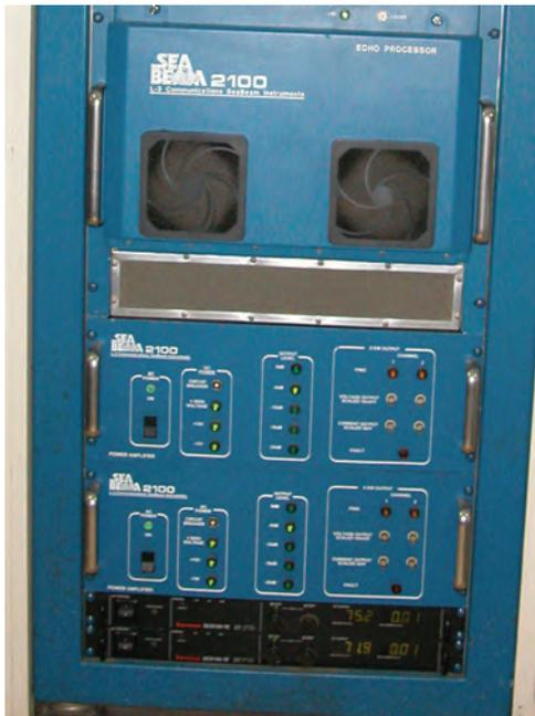
Figure 6.12: SeaBeam 2120 system electronics cabinet.
