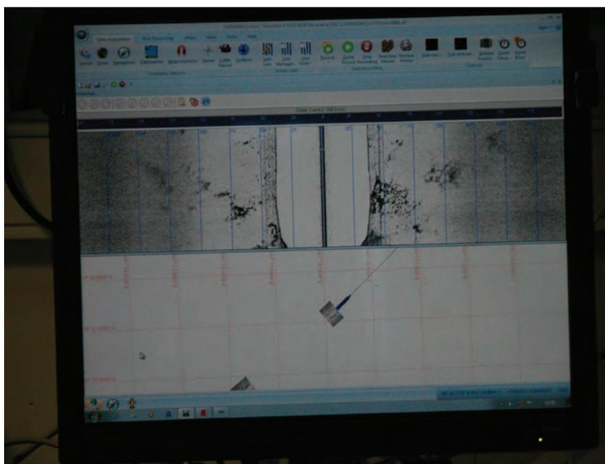
Figure 6.19: Acquisition of side-scan sonar data using the SonarWiz Map software.
