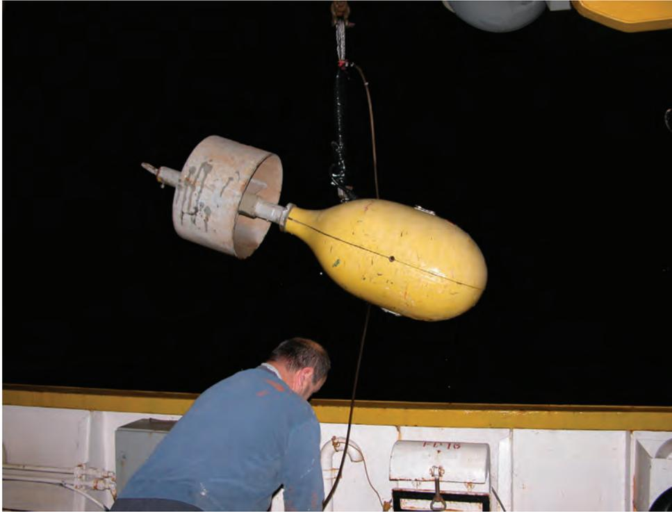
Figure 6.16: Deployment of the 3.5kHz sub-bottom profiler tow fish over the left side of R/V AEGAEO during the Farasan cruise.
