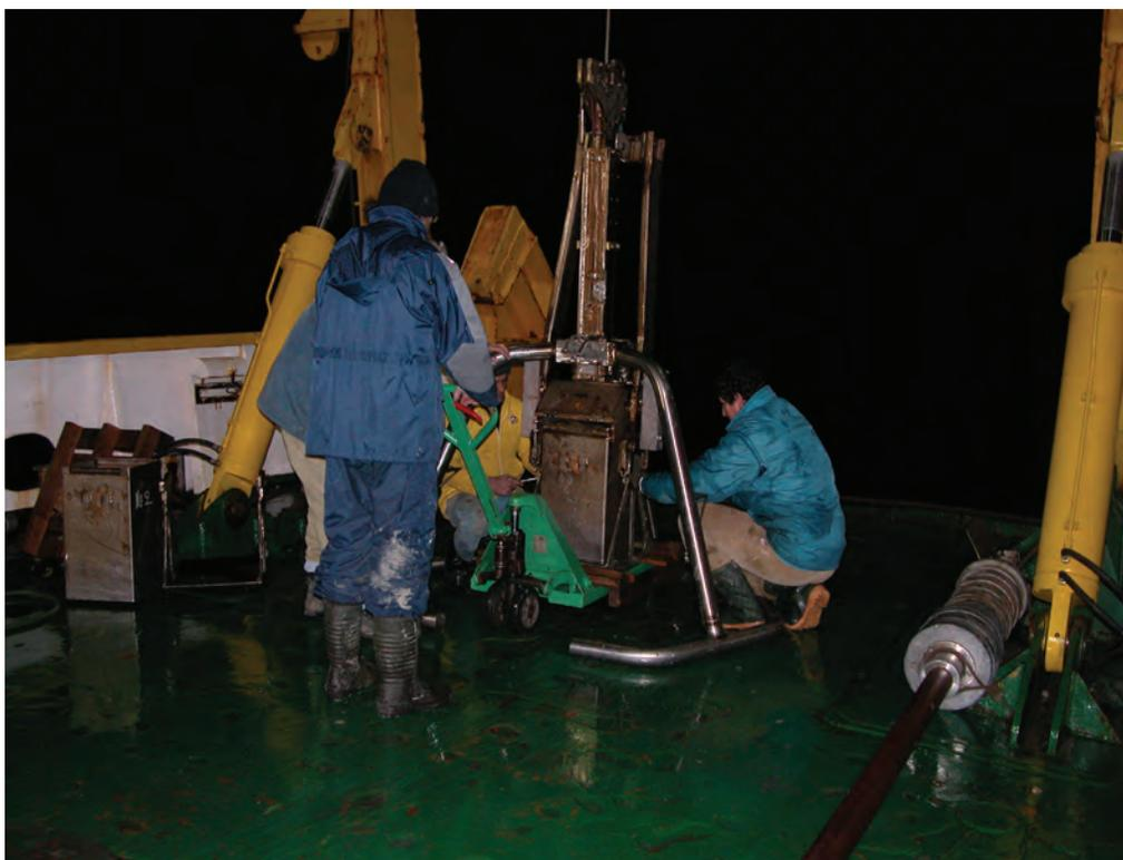
Figure 6.23: Box corer deployed through the A-frame at the stern of R/V AEGAEO in the Farasan area.
