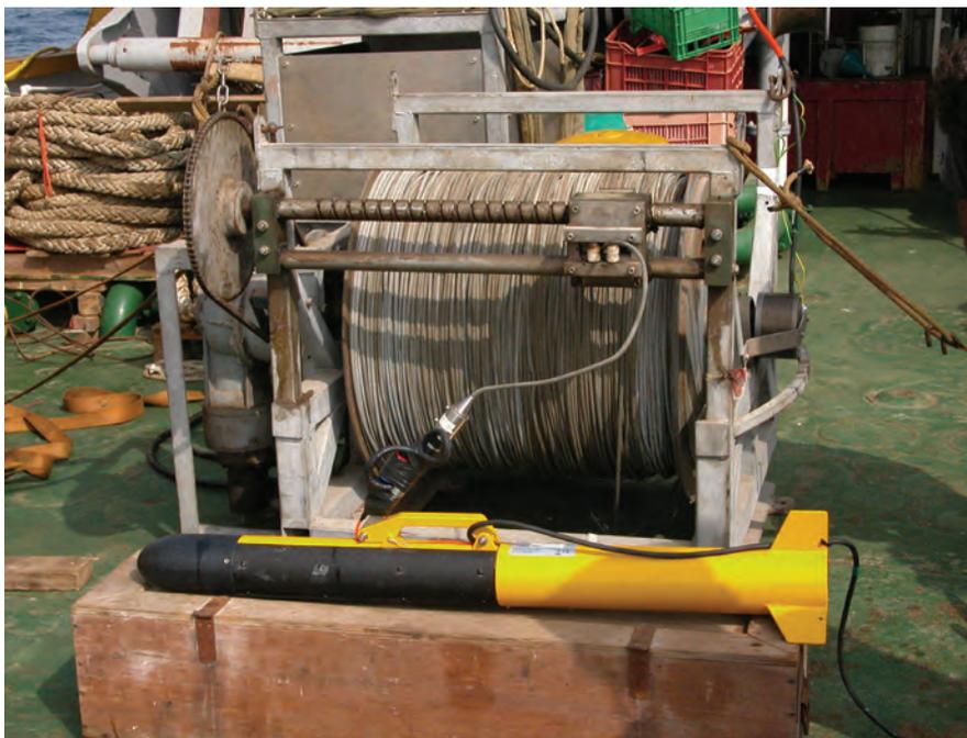
Figure 6.18: Side scan sonar tow-fish and tow-cable winch on the working deck of R/V AEGAEO during the Farasan cruise.
