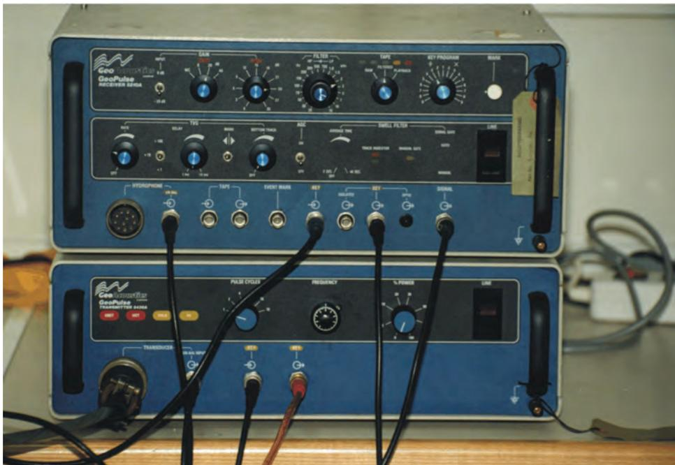
Figure 6.17: Receiver and transmitter (GeoAcoustics Ltd. GB) devices used as deck units for controlling the 3.5kHz acoustic signal.
