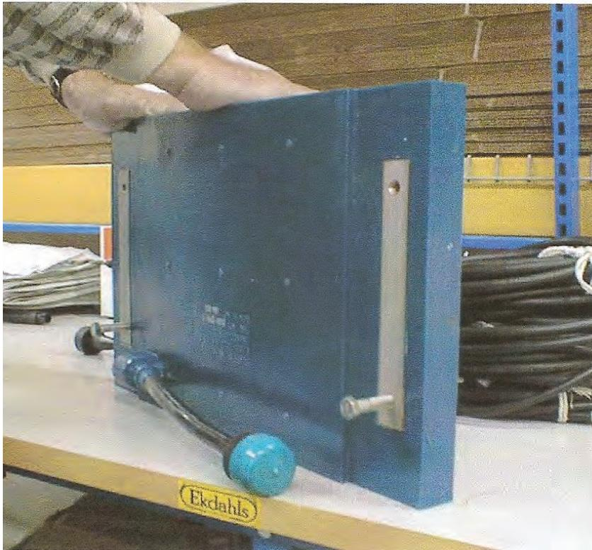
Figure 6.10: Hydrophone of the SeaBeam 2120 multi-beam system.
