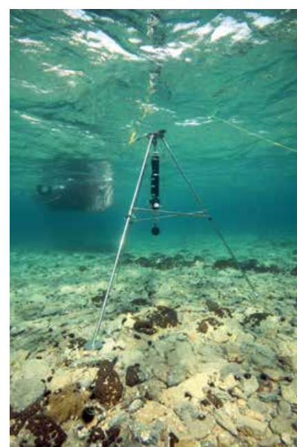
Fig. 6.2 Side scan sonar image (400 kHz), obtained in 2-4 m water depth of the submerged prehistoric city of Pavlopetri in Greece. Blue lines highlight the remains of the walls of the buildings and roads. (Sakellariou et al. , 2011) The image on the right shows a sector-scanner (Kongsberg MS1000) mounted on a tripod, and deployed in the centre of the ruins at Pavlopetri. The sector scanner projects sound at 750 kHz, and rotates in the tripod to build up a radial picture.
